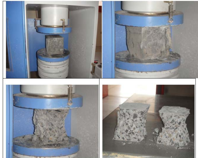
Fig. 2: Test procedure for compressive strength test
